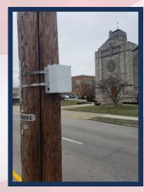
Armadillo device for covert traffic surveys. This device can gather traffic statistics from multiple lanes and travel directions. Its small size allows for trouble free setup and is hardly noticeable while mounted for data collection. The radar can collect traffic data for weeks on a single battery charge and can withstand various types of weather conditions. So far, this device has been used to conduct studies in four different locations.
